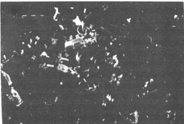
Fig. 15. SEM of rice straw ash obtained after burning the acid-leached (1 N HCl) rice straw sample in the muffle furnace at 600°C.
